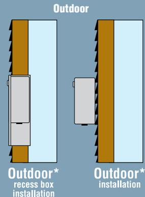
\*Outdoor units do not require venting materials. Venting details, including clearances and diagrams can be found in the "Use & Care Manual" of Rheem indoor tankless water heaters.
